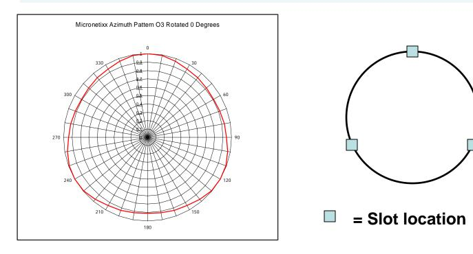
The Omni-directional antenna pattern needs a bigger pylon diameter to get the proper current flow around the pylon. For a UHF slot antenna, the minimum diameter is 6 inches (15 cm) and can vary to 16 inches (40 cm.) for large top mounted pylons. When larger top mounted antennas come into play the slot count can be increased to 4 or 6 slots per bay. As the slot count per bay goes up on a top mounted antenna, the thickness of the pylon needs to go up to keep the pylon rigid.
