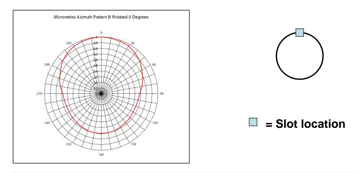
The azimuth plot above is an Omnioid antenna. To the right is a birds eye view of the antenna pylon, with the location of it's column of slots. The antenna has an average azimuth gain of 1 (0.0 dB), or if thought of as a directional antenna, the azimuth gain is 1.7 (2.30 dB). Along the back sides of the pattern, the field value falls to about 65% of peak, and is at 70% of peak field at 180 degrees opposing the slot location.
