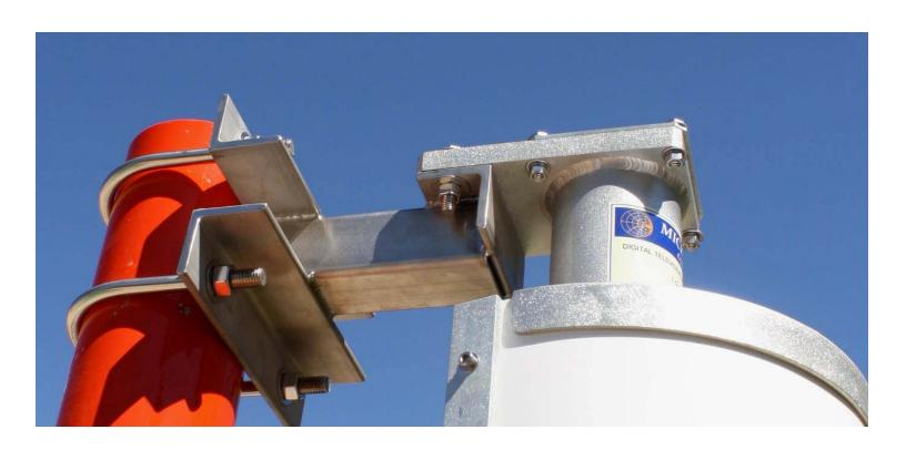
As antenna patterns and frequency of operation varies, so does the optional distance from the tower change. With our modular approach to bracket construction, we can tailor the bracket length for best antenna performance. On heavier antennas, we use triangulated brackets. The brackets can be designed for either a leg mount, or across a tower face.
